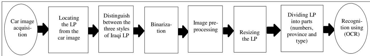
Fig. 3. The main stages of the LPR system
