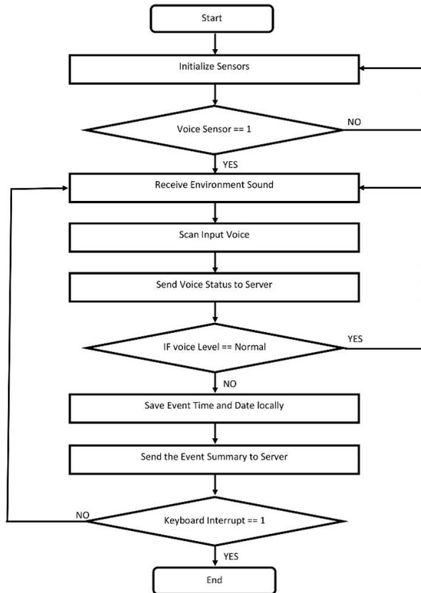
**Figure 2.** Block diagram of the complete system. The inputs of the system are the sound acquisition that goes through the T-Bone GC100. Raspberry-Pi-3 Model B, is in charge to remove power line noises. Then it analyzes the signals and in case of abnormal situation it sends the status to the server.
