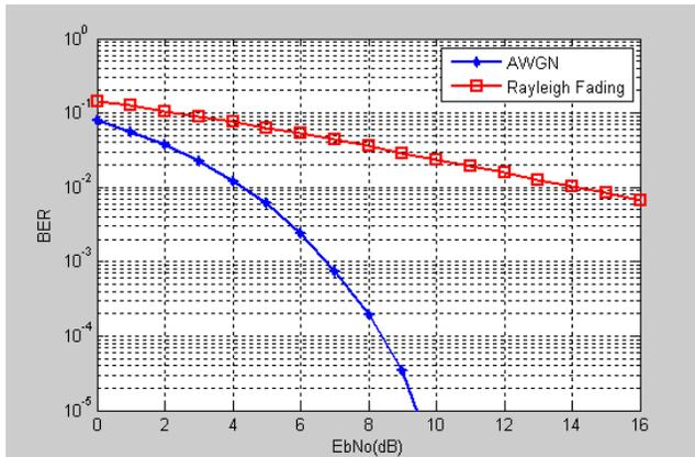
Figure 8. BER Vs. Eb/No Simulation Comparison for OFDM over AWGN & Rayleigh channel
