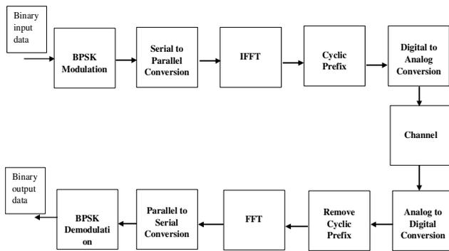
Figure 1. Basic OFDM Transceiver
