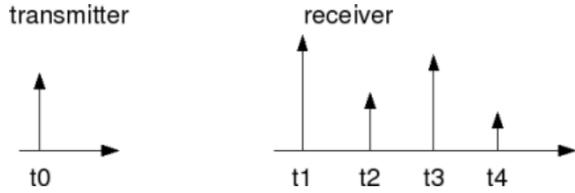
Figure 5. Impulse response of a multipath channel
