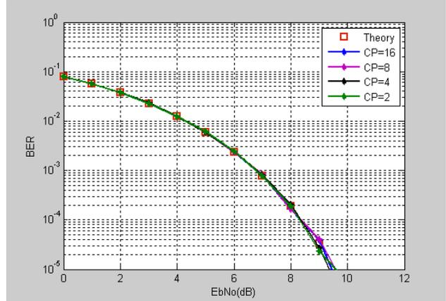
Figure 6. BER Vs. Eb/No for OFDM over AWGN channel with different CP
