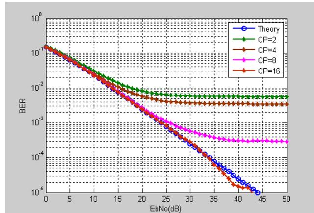
Figure 7. BER Vs. Eb/No for OFDM over Rayleigh channel with different CP
