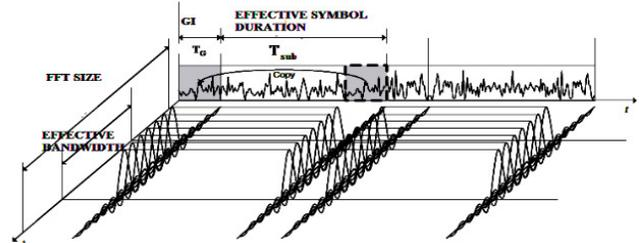
Figure 3. Time/Frequency domain OFDM Symbol with CP
